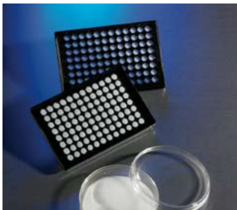
« Corning 96-Well plate with Ultra-Web nanofiber surface
