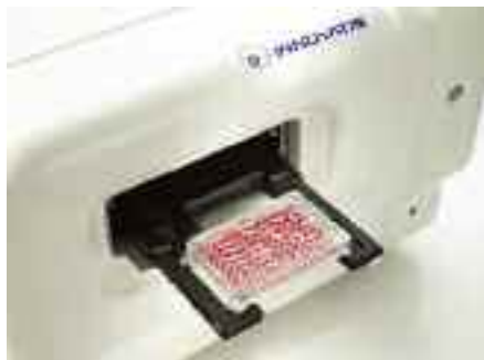
Cellavista from innovatis, combines brightfield and fluorescence optic capabilities.
